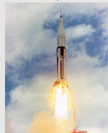
AS-202 Suborbital flight to Pacific Ocean splashdown. CM heat shield tested to higher speed.
