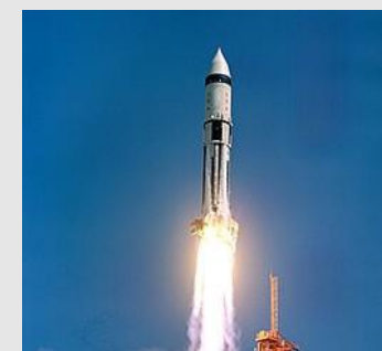
AS-203 Uncrewed flight of the Saturn IB rocket to test rocket stage restart capability.
